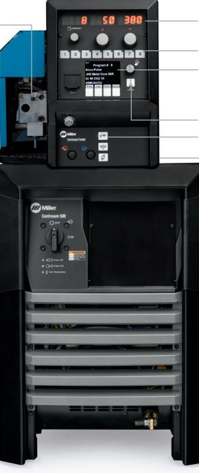
**Display and controls** for program select, volts/arc length and wire feed speed
